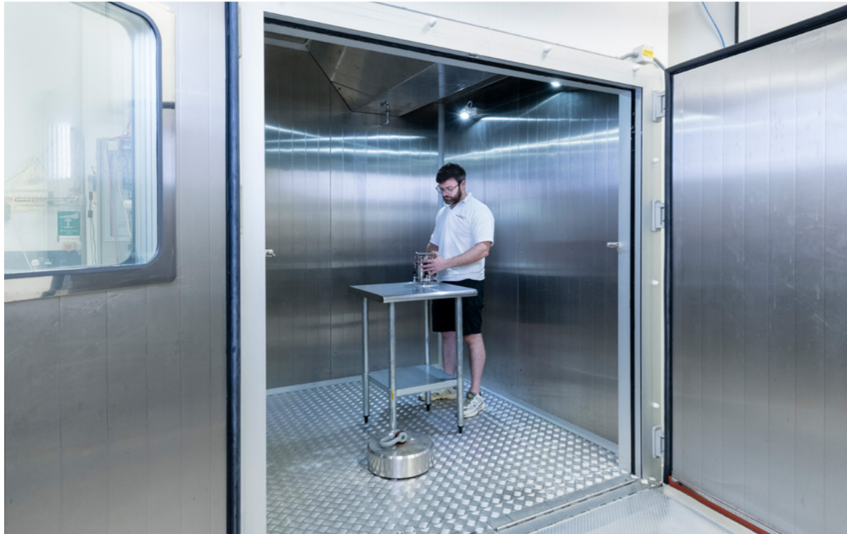
Large (2.1 x 2.1 x 2.6m) chamber (mini-satellite sized) with a wide temperature range of -30°C to +70°C, with nitrogen purging available.
